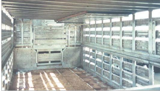
■ Interior view of bottom deck of double decker trailer. Besides the 3" I beams protruding below the ceiling, there is a ramp that is stored on the ceiling.
