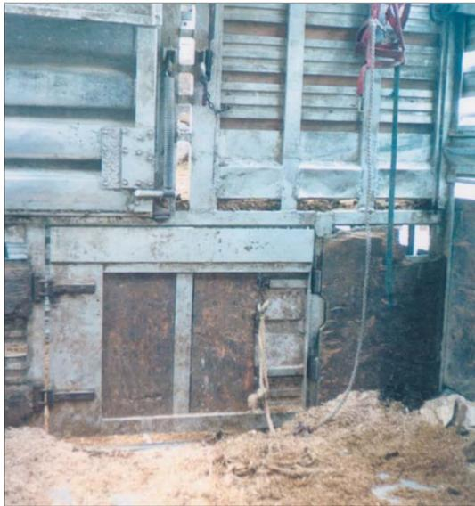
■ Above: "Doghouse" area of trailer. Ramp to top deck is on the left. Door in middle adjacent to floor opens to bottom deck.
