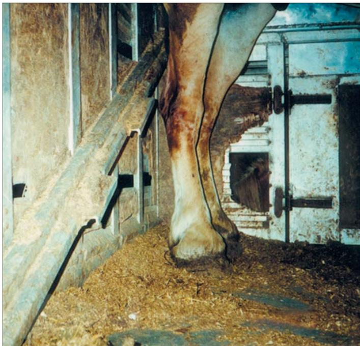
■ Above: Horses inside the “doghouse” area of a double decker. Note the exposed metal floor and the hole in the wall behind the horse’s leg, (horses are at risk for injury if they were to kick or paw and the leg would become caught in the opening.) Also note the slanted, sharp metal protrusion on wall behind horse’s leg, which supports the ramp to top deck when it is in the “down” position.
